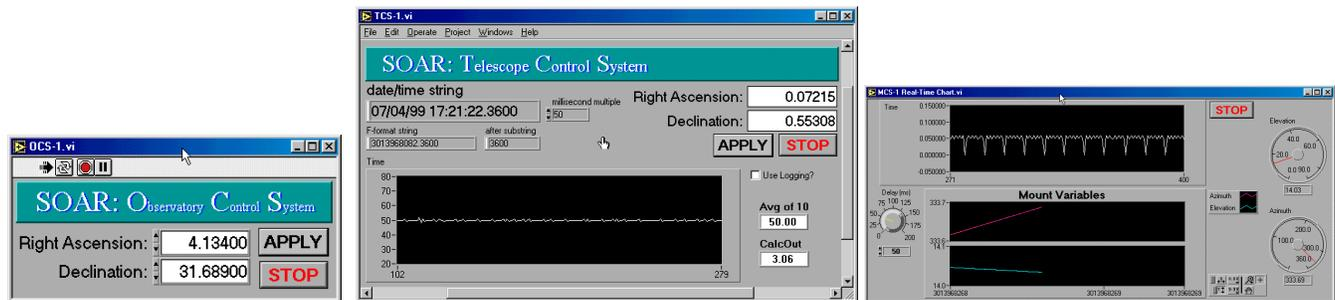
**Figure 2.0** First demo GUIs. The module layout of the first TCS demo implemented in LabVIEW and "C" for the SLALIB function calls.
