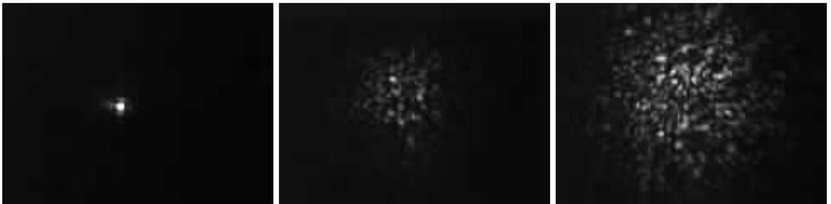
**Figure 2.** Image of a monochromatic point source with the simulated telescope. These graphs show, from left to right, the degradation of the image quality when putting 0, 1 and then 2 phase plates in the beam. The aperture is about  $8 \text{ mm}$  on the phase screen for a  $r_0 \approx 500 \mu\text{m}$ . Different intensity scale for different configurations improves the contrast.  $\lambda = 633 \text{ nm}$ .
