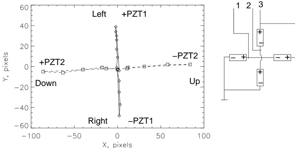
Figure 3: LLT pointing reaction on changing voltages on the tt platform (in auto-collimation). Up-left directions correspond to beam displacement on the sky, XY – to ATP pixels. The scheme on the right shows the connection of four piezo actuators to the driving voltages on PZT1 and PZT2 (variable from 0V to 100V) and PZT3 (constant 100V), with the common line grounded.
