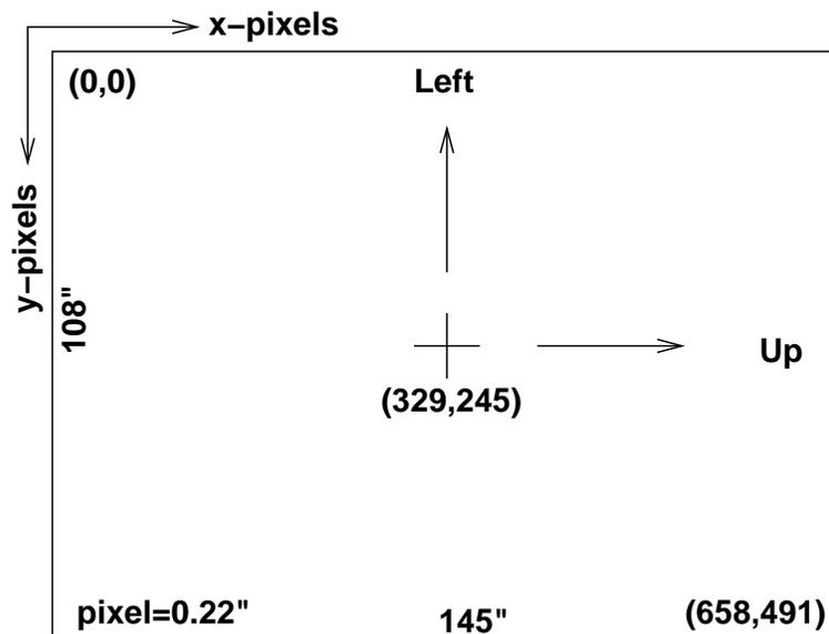
Figure 2: ATP field as displayed on the screen with directions on the sky and some useful numbers. When SOAR points near the meridian to the North of zenith, the SOAR offset to the North (down) moves the star right, offset to the East (right) moves the star up. The North/East directions are reversed when SOAR points near the South Pole.
