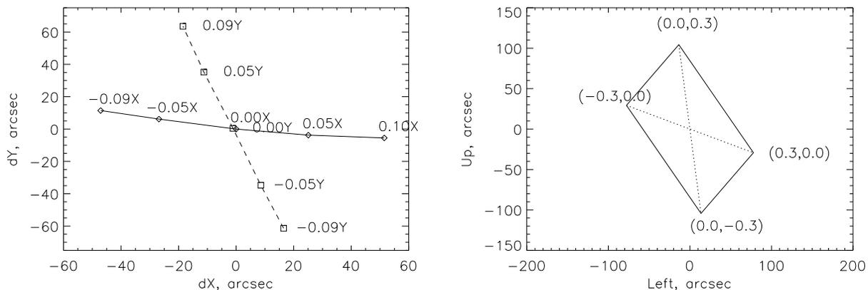
Figure 4: Left: motion of the spot on the sky (Y up, X left) when M1 is actuated in X and Y. The commanded M1 displacements in X and Y (in mm) are indicated near the curves (data from SDN 2323, Sect. 4.6). Right: range of the LLT pointing adjustment by M1 motions. The numbers indicate the (X,Y) coordinates of M1.
