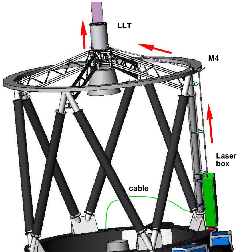
Figure 9: Beam transport from the laser box to the LLT.
