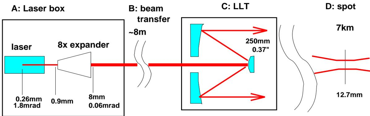
Figure 8: Path from the laser to the LLT. The beam diameter  $2w$  and divergence  $2\theta$  (both at  $1/e^2$  level) are indicated.
