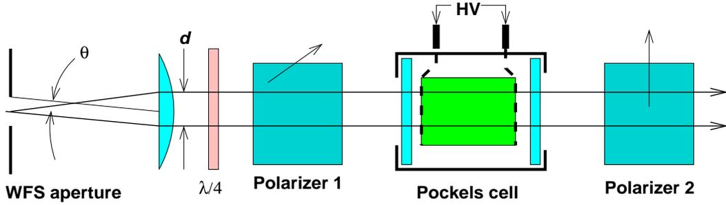
Figure 5: Pockels-cell shutter. An electro-optic crystal KD\*P is placed between crossed polarizers. No light is transmitted until a voltage is applied during the range gate time  $\Delta t$ . The light entering the shutter is converted from circular to linear polarization by the  $\lambda/2$  plate.
