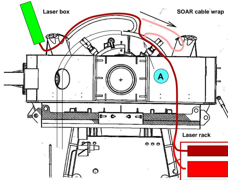
Figure 10: Suggested cable path from the laser to its cooler and electronics installed in a thermal rack.
