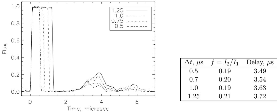
Figure 6: Light pulse transmitted through QX1020 Pockels cell with crossed polarizers, He-Ne laser, 4 kV pulse amplitude, for varying length of the drive pulse (in  $\mu s$ ). The relative intensity and delay of the ringing after-pulse are listed in the table.
