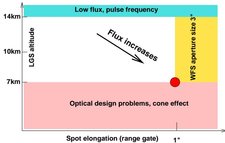
Figure 3: Trade space of the SAM LGS parameters – spot distance from the telescope (altitude)  $H$  and spot elongation  $\alpha$ . The red circle depicts chosen parameters.
