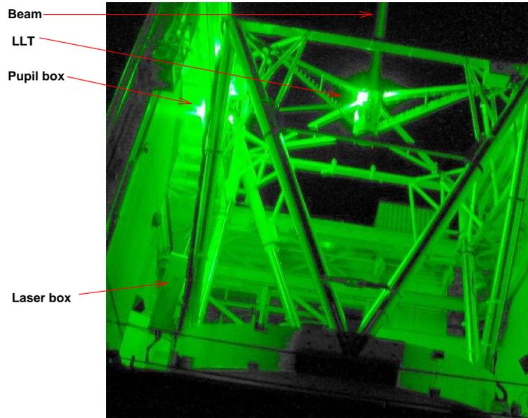
Figure 2: The Rayleigh LGS system at MMT, as viewed from outside of the dome. The beam path from the laser box to the LLT is in the air.
