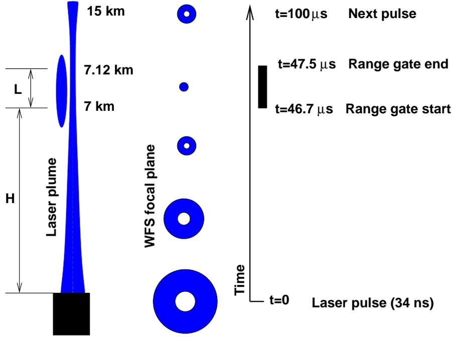
Figure 1: Propagation of the laser pulse (“bullet”) in the atmosphere and range-gating. The “donuts” depict defocused images of the laser spot in the wave-front sensor (WFS) at different moments.
