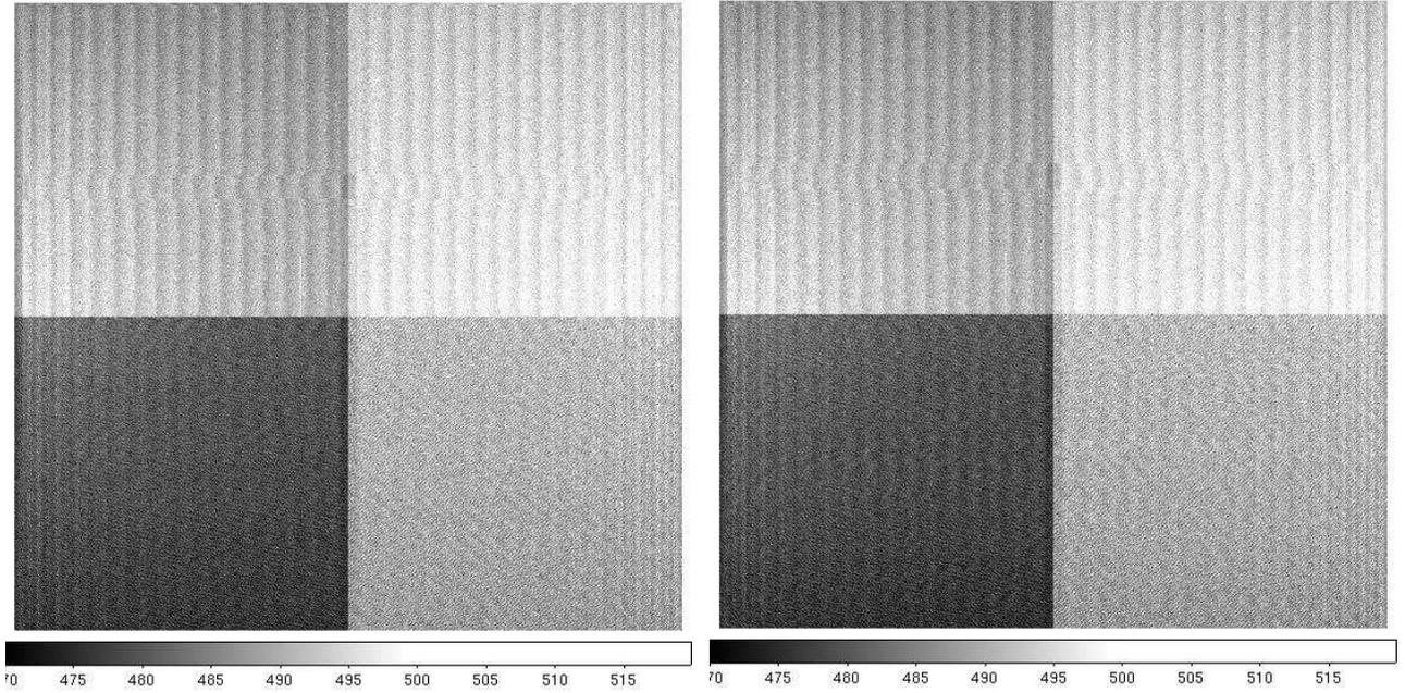
Figure 4: Two full bias frames with 4x4 binning in the fast readout mode.
