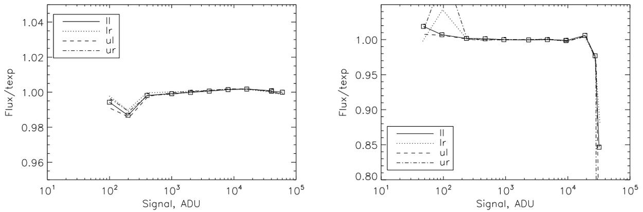
Figure 7: Linearity of the CCD response in the normal (left) and fast (right) readout modes determined with the LED. Curves for all 4 quadrants are plotted.
