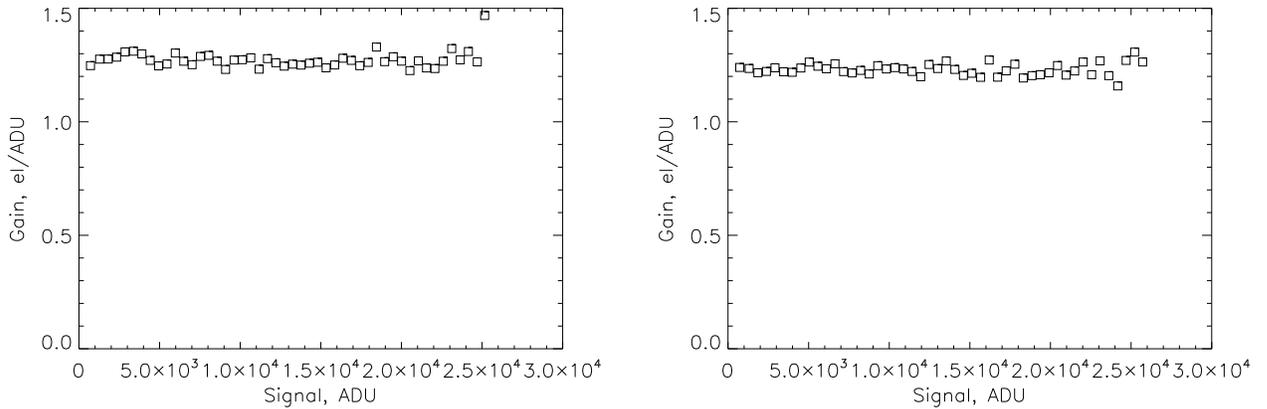
Figure 5: Gain vs. signal level for quadrants 0 (left) and 2 (right) computed from the ratio of two quartz exposures `chi120325.1008.fits` and `chi120325.1009.fits`.
