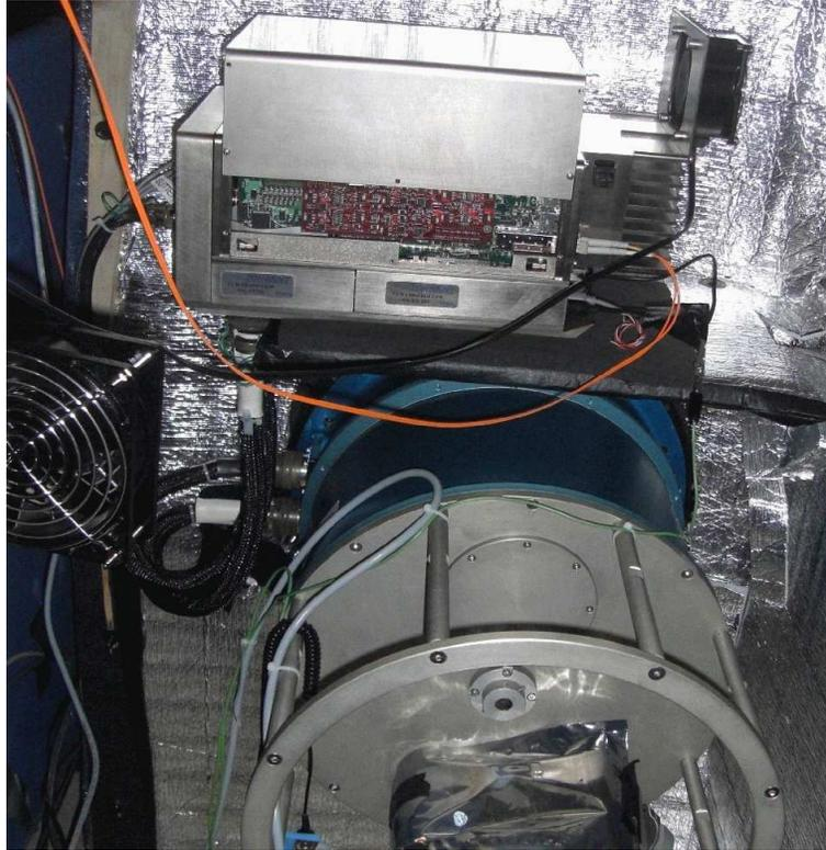
Figure 1: Torrent controller is installed on a small shelf above the CCD dewar and connected to it by two 40-cm cables. The controller is half-opened and air-cooled to prevent power supply failures caused by overheating.
