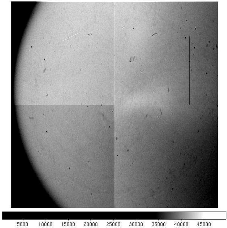
Figure 6: Quasi-uniform illumination by the LED (image LED0012.fits, 10s, 4x4 binning, normal mode). The bias and overscan are removed, but the gains are not applied, causing discontinuity between the quadrants.
