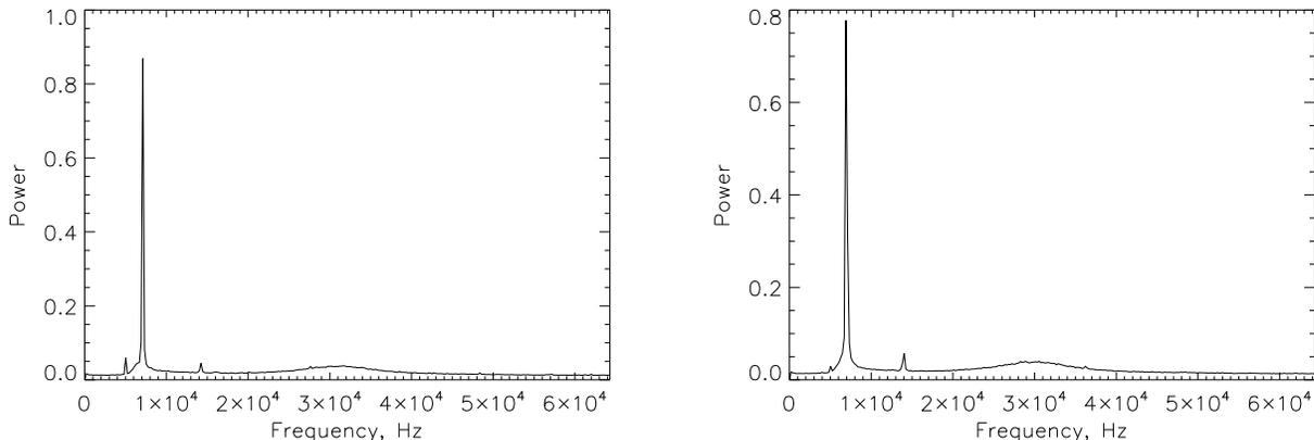
Figure 3: Power spectra of readout noise in quadrants 0 (left) and 2 (right) of the bias frame `chi120325.104.fits`, assuming pixel frequency of 129 kHz.
