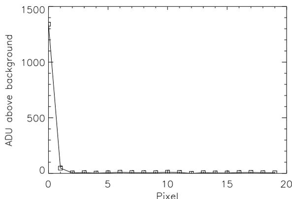
Figure 8: Evaluation of the vertical CTE from the combined trail of cosmic particles. The plot starts at the last bright pixel. Data of February 14, 2012.
