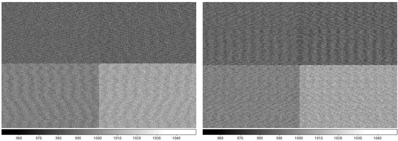
Figure 2: Central fragments of bias frames with binning 3x1 (left, `chi120325.1049.fits`) and 4x4 (right, `chi120325.1058.fits`) in the normal readout mode.
