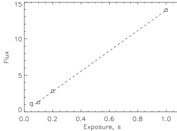
Figure 4: Flux of selected Th-Ar line vs. exposure time.
