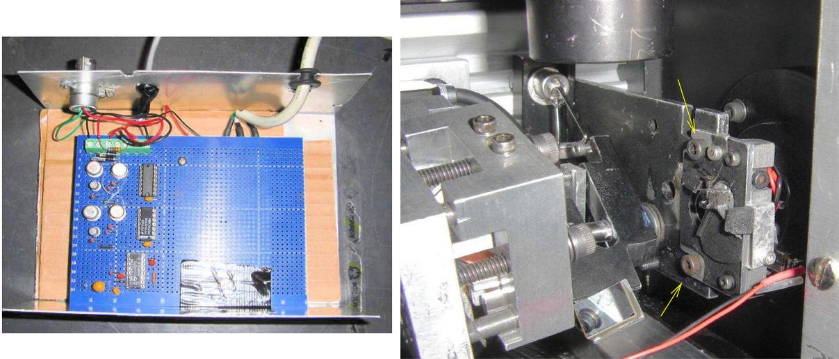
Figure 3: Left: driver in its open box. Right: shutter installed in CHIRON. Yellow arrows show the two screws used to fix the shutter.
