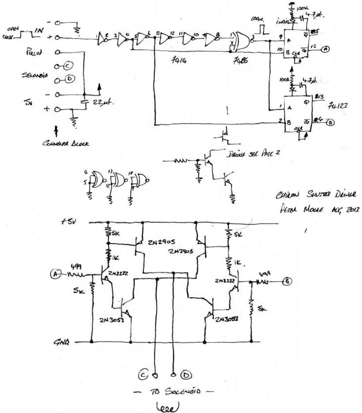
Figure 2: Electronic schematics of the new driver.
