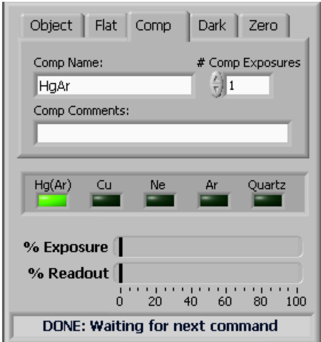
The wavelength calibration lamps normally used with the Goodman spectrograph are: HgAr, CuHeAr, Ne, and Ar. An Fe lamp is also available.
