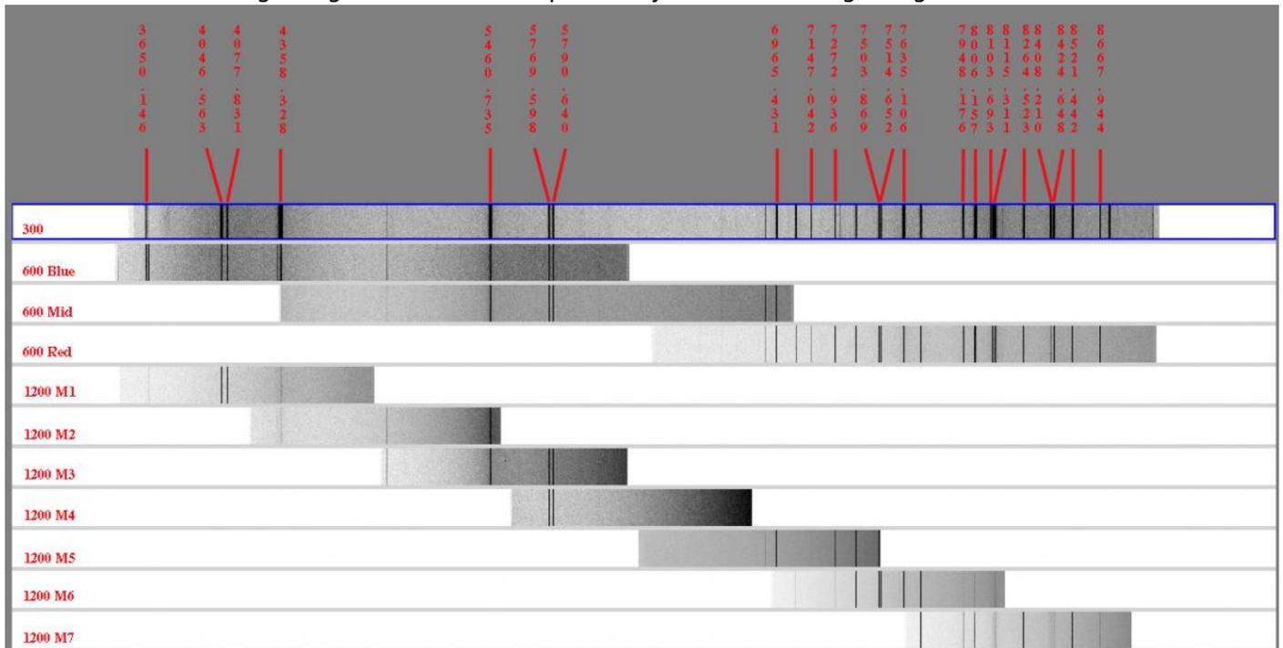
In the following table containing plots of the comparison lamps made with various gratings and setups. This library of comparison lamp spectra will be expanded and updated to make it include most, if not all of the setups available with the instrument.
