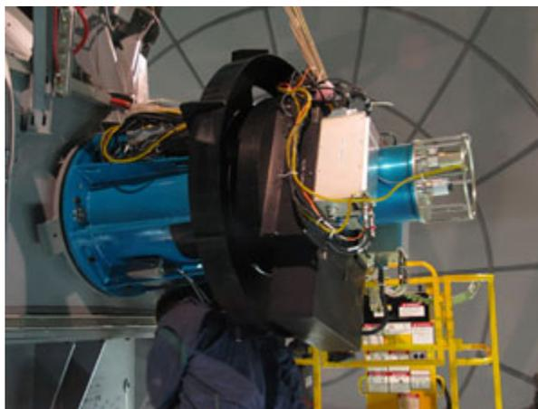
*Figure 4: The SOI system mounted on one of the bent-Cassegrain foci of the SOAR Telescope. The dewar containing the 2 CCDs is the smaller blue cylinder located on the right. The SDSU Leach controller is the silver box located in front of the dewar.*
