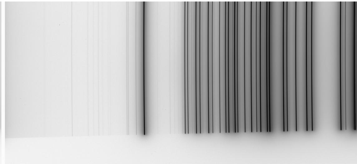
Figure 3: Spectrum of a HgArNe comparison lamp taken with same setup as that of Figure 2 above. The spectral lines toward the red (right) are cutoff as the image of the spectrum falls off the upper part of the detector.
