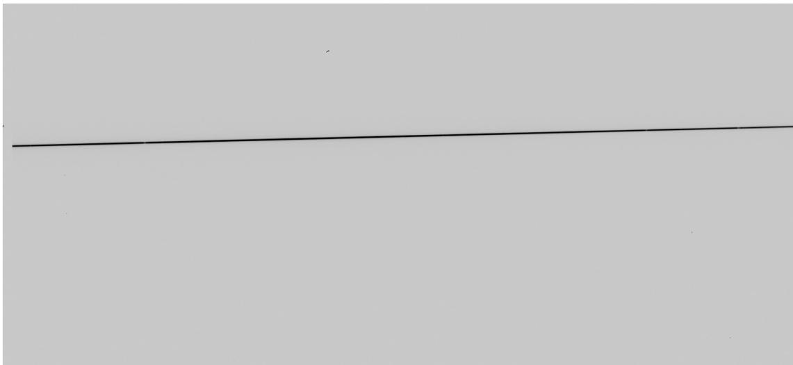
Figure 2: Spectrum of the standard star HD 60753 obtained on Feb 12, 2020 with the 600\_old grating, 2x2 binning, 1" long slit and MID setup (435-702nm). The grating was in its previous position within the holder, as shown in Figure 1. The vertical difference between both ends of the spectrum is 51 pixels, equivalent to 2.5%.
